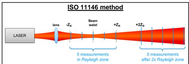
**Figure 1:** In the ISO 11146 method, the beam width must be measured along the optical axis at 5 various positions distributed within the Rayleigh length and 5 others beyond two times the Rayleigh length. At each location, 5 measurements have to be done. The beam width is calculated based on second order moment. A hyperbolic fit then provides the  $M^2$  value.
