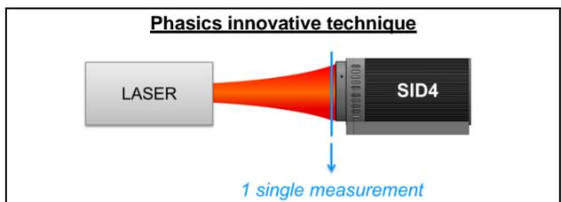
**Figure 2:** Phasics' sensor is placed anywhere along the optical axis where the beam fits the sensor aperture. Therefore the sensor can handle rapidly diverging beam for which the diameter at a distance above 2 Rayleigh lengths may be too large to be measured with the ISO 11146 method.
