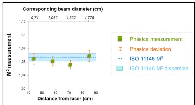
Similar measurements were realized for a laser of a  $M^2$  far from 1. Again, the results of both techniques match. These two series of measurement proved that the **Phasics’ method for  $M^2$  measurement is completely in agreement with the ISO 11146 standard** both in terms of expected repeatability and accuracy.
