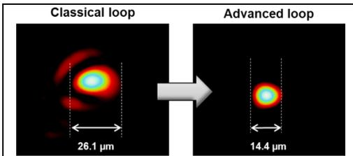
3. *In this example, the focal spot size of a  $f/5$  beam is improved by 45% with Phasics advanced process*
