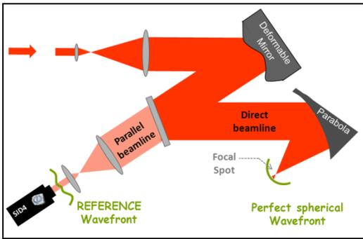
2. *Step 2: the wavefront measured in the parallel beamline is saved as a reference*
