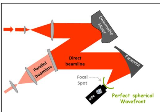
1. **Step 1:** the mirror actuators are moved so as to obtain a perfect spherical wavefront just after the focal spot
