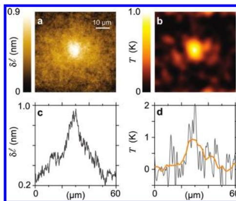
**Figure 4.** (a) Raw thermal-induced OPD image obtained on a quasi-hexagonally ordered array of gold nanoparticles (see Figure 3a). (b) Processed temperature distribution (smoothed using a 10-pixel Gaussian function). (c) Cross section of image a. (d) Cross section of the raw image (b) without smoothing (dash line) and with smoothing (solid line).
